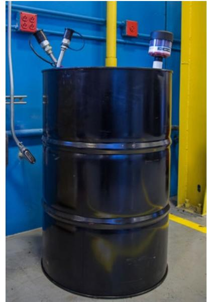
Figure 5. Desiccant breather installed on a drum.
